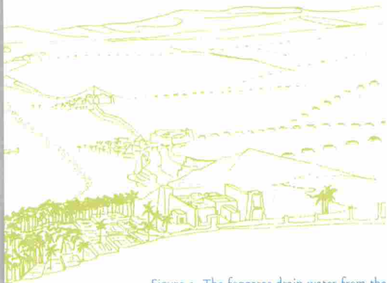
Figure 1. The foggaras drain water from the groundwater sources to the oases. Vertical wells along the underground galleries provide aeration and allow for maintenance. (Illustration: Concetta
